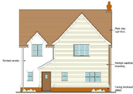
FRONT ELEVATION 1:100 ELEVATIONS
